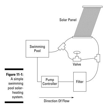
When the valve is closed, water runs exclusively through the solar collect or panel, heating the water. As you open the valve, water flows less and less through the collector panel because the path through the valve is so much easier. In this way, you can adjust how much heat is going into your pool. In the middle of summer, you may not want any additional heat.
