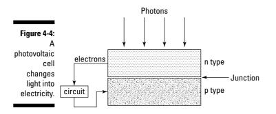
Photovoltaic arrays are nothing more than huge matrices of interconnected semiconductor sandwiches. The color appears shiny blue. Usable PV systems are comprised of all sorts of equipment that protects the user from electrical shock, stores the electricity in battery banks, and converts the direct current (DC) into alternating current (AC), which is what people use in their houses. But at the heart of each system is a simple conversion process like that shown in Figure 4-4.
