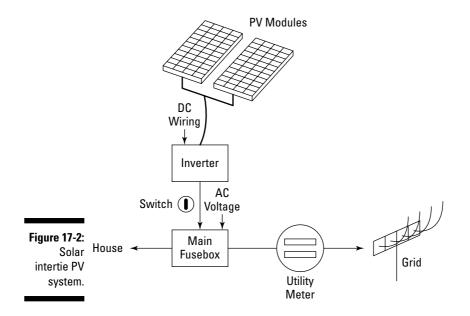
The following sections describe the various parts of a solar PV system.
