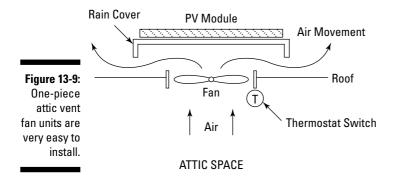
One-piece attic vent fans are very simple to install; you don't even need to go into the attic space. Simply cut a round hole in your roof, pull the shingles back, slide the unit up under the shingles, and drop it into the hole. Seal for weatherproofing, and you're done.
