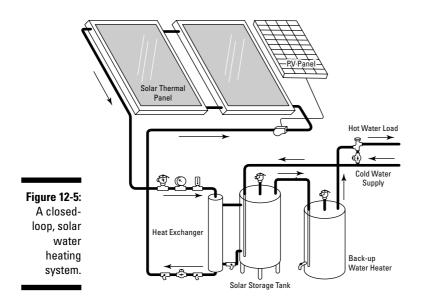
The flat-plate collectors can be mounted in almost any configuration, at great distances from the exchanger. The closed loop is always full of fluid, so the pump pressure requirements are much easier than those for a drainback system.
