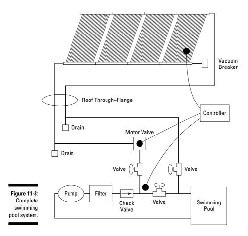
Piping is almost always 2" PVC. Keep  $90^{\circ}$  bends to a minimum because they increase the resistance to water flow, which makes the pump work harder.
