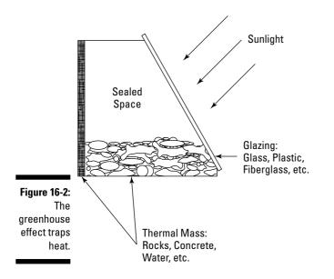
Sunlight enters the enclosed space through the glazing (window) and then gets absorbed and stored as heat energy. The heat is then constrained to stay in the enclosed space via the same glazing's insulation properties, plus insulation in the walls. You can enhance the greenhouse effect by increasing the amount of radiation the window allows to enter while maximizing the glass's insulation against heat.
